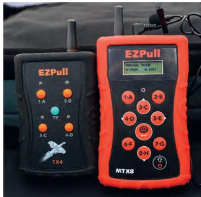
true pairs by simply pushing the TP button in the center, then the numbered trap release buttons. The buttons are raised with a distinct 'nipple'. They can be felt through gloves and cold weather shooters will love them. The TX4 would be great for a super sporting setup, new style FITASC or any four-trap sporting layout.
