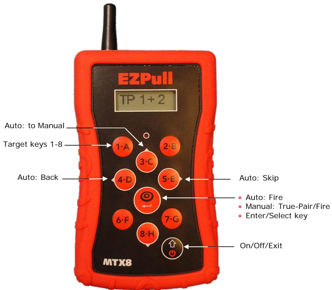
White circle/arrows on a key means it is also used for navigation, modification and selection
