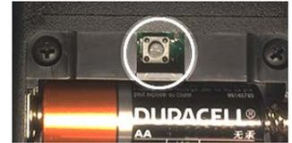
2. Exit Setup Mode: When in Setup mode, press and release the setup switch above the batteries. Unit will go directly to Release mode, ready to release targets.
