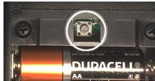
2. Exit Setup Mode: When in Setup mode, press and release the setup switch above the batteries. Unit will go directly to Release mode, ready to release targets.
